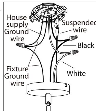
**5.** Use the suspended wire to hang the fixture as shown for wiring connection.
