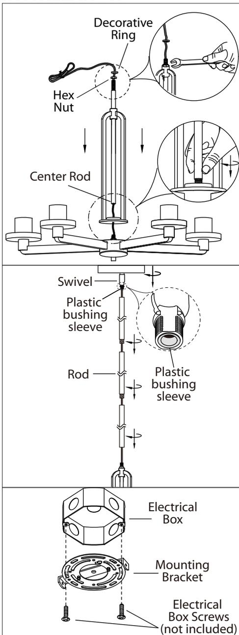
**1.** Assemble the fixture by screwing the center rod to the threaded tube in the center of the fixture.
