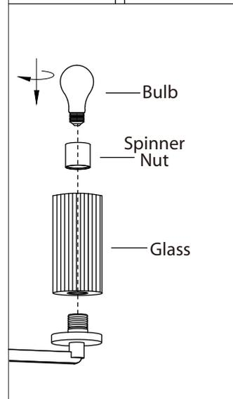
**9.** Remove spinner nut from socket. Position glass on lamp and secure with spinner nut. **(Please check the glass before installing for any cracks. Do not overtighten the spinner nut to attach the glass to the fixture.)**
